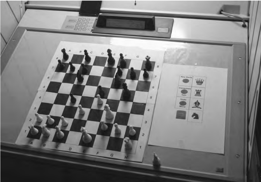
Figure 7.5: Dutch researchers showed that they could quickly replace the firmware ROMs in the Nedap ES3B DRE to tamper with votes ... or make it play chess [263].
