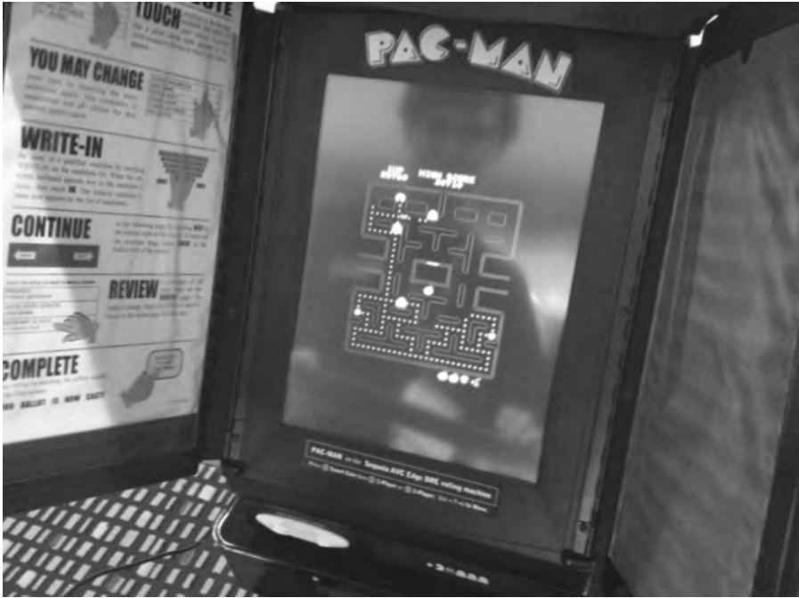
Figure 7.4: Voting researchers converted a surplus Sequoia AVC Edge DRE into a working PAC-MAN machine to show how easily its software could be modified [281].
