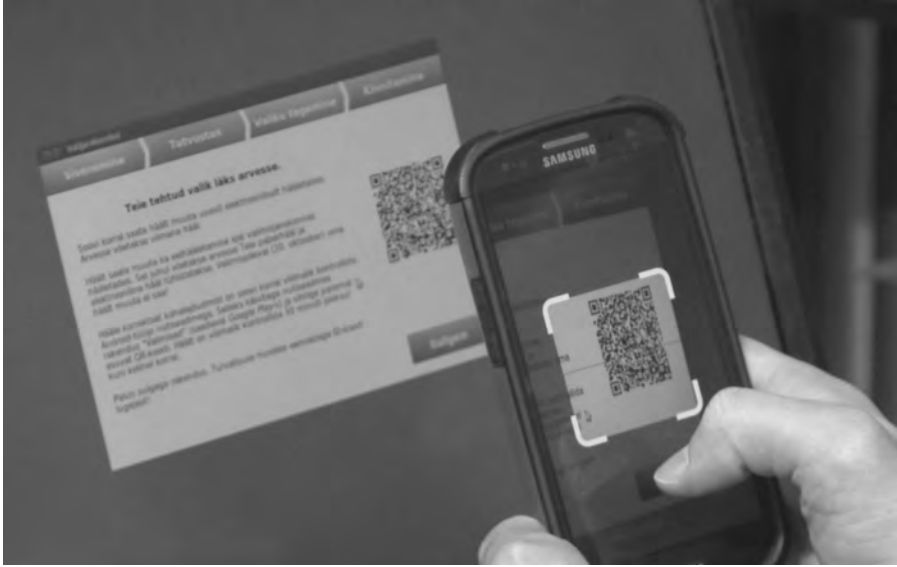
Figure 7.12: Voters in the Estonian Internet voting system can confirm their votes by scanning a barcode with a smartphone app [535]. Researchers showed that this mechanism could be bypassed by malware on voters’ computers or election servers.
